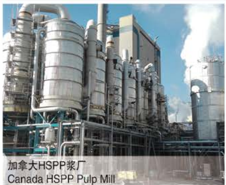
板式降膜蒸发器 Plate Falling Film Evaporator
