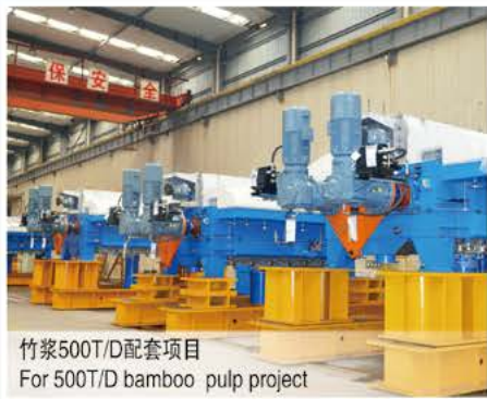
机械驱动双辊洗浆机 Wash Press by Mechanical drive
