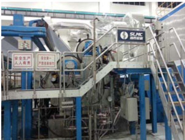
Figure 4 An example of transformation to film transfer sizing machine
