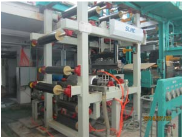
Figure 5 The pilot test curtain coating machine developed by SLMC and CNPPRI
