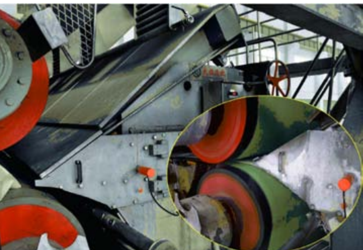
Figure 1 Headbox with dilution water developed by Henan Dazhi Paper Machinery Co., Ltd.
